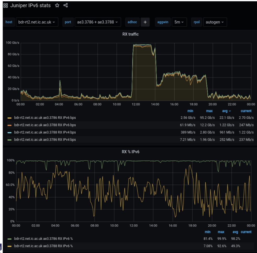
Figure 1 — Imperial monitoring shows the two-hour period where the 100G link was filled and where 100% of the LHCONE traffic was IPv6.
