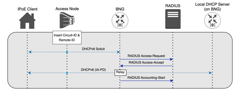
Sky uses port-based authentication for subscribers, using a string inserted into DHCP messages by Openreach's access nodes. Specifically, into the Remote-ID options, DHCPv6 Option 37 and DHCPv4 Option 82 sub-option 2.
